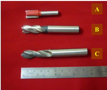
Figure 1. Various types of drilling cutters of 10 mm diameter: (A) router; (B) end mill cutter; (C) twist drill. This figure is published in color in the online version.
